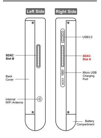
SDXC Slot A and CF card slot cannot be used concurrently. The UDMA3 can only access one of the 2 card slots at any point of time.
