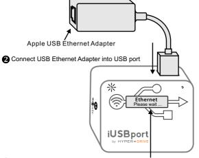
If the Ethernet adapter is recognized, iUSBport will display 'Ethernet' on the LCD. Once iUSBport gets an IP address, it will switch to router mode and a router icon will appear on the LCD.
