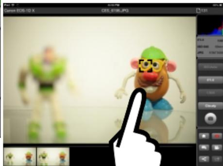
**If you trigger the shutter during AF driving, camera will stop AF driving and capture image immediately. Therefore, you will get an unfocused image.**
